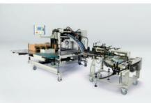
Omega Pack is a fully automated case and 4 & 6 corner work as well as many carton production on Omega folder gluers. Omega Pack can pack up to 4 rows and 4 layers, requires a single operator and takes 10-15 minutes to make ready. It handles straightline
