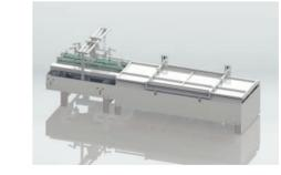
Omega Turnpro is a separate module which turns the direction of the carton flow by 90 degrees on the folder gluer and is a significant value-add feature. It is developed for producing specific cartons, such as multi-pack beverage carriers, confectionary, e-commerce and cosmetics boxes for high speed production in a single pass.
